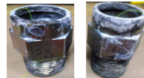
Samples after 400h tested according to ISO 9227 NSS
